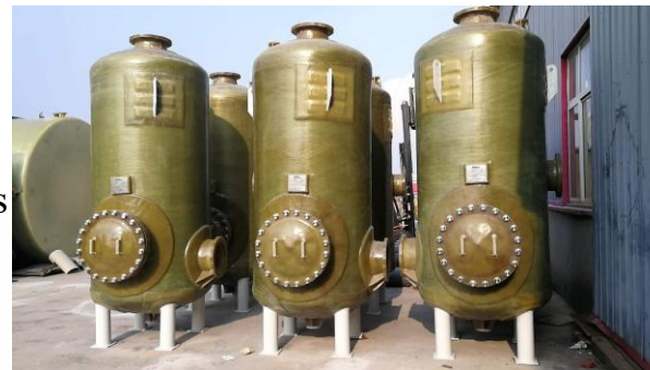
Vacuum receivers, storage tanks and related piping for Westech/Jacobs Morocco project
