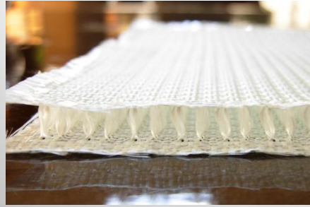
3D vertical weave fiberglass
