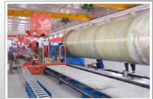
One of 29 automated pipe winders
