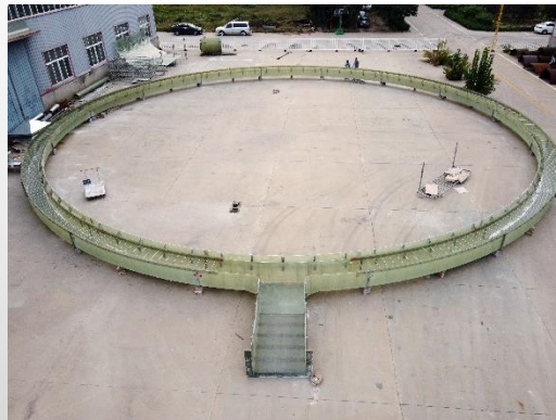
Two 120' diameter trough, weir and drop out systems for Puerto Rico
