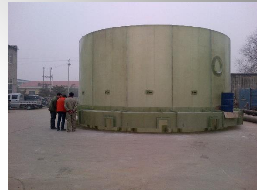
4 feedwell and reaction wells sets with troughs and piping for 85' dia. clarifiers in Australia
