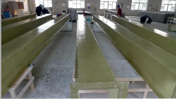
4 feedwell and reaction wells sets with troughs and piping for 85' dia. clarifiers in Australia
