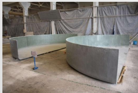
Heads fabrication and cutting
